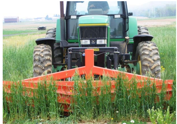
Figure 2. Picture of a Penn State roller/crimper rolling a rye cover crop.
