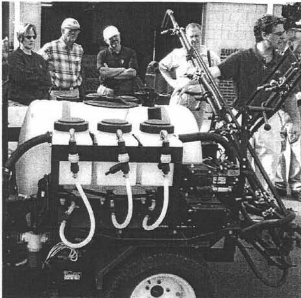
In 2002, the Toro Company and Raven Industries (South Dakota) donated an injection sprayer that could apply small quantities of materials which greatly aided treating the IPM-managed greens.
